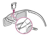
2 Replace the battery with a new one. After that, be sure to insert the battery case until it locks in place again.
