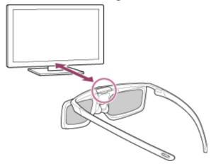
The Active 3D Glasses turn on and registration starts (the () (Power) button/indicator blinks green and yellow). When registration is finished, a message appears in the TV screen for 5 seconds, and the indicator lights up in green for 3 seconds.
