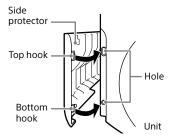
2 Secure the side protector to the unit with the supplied screw.
