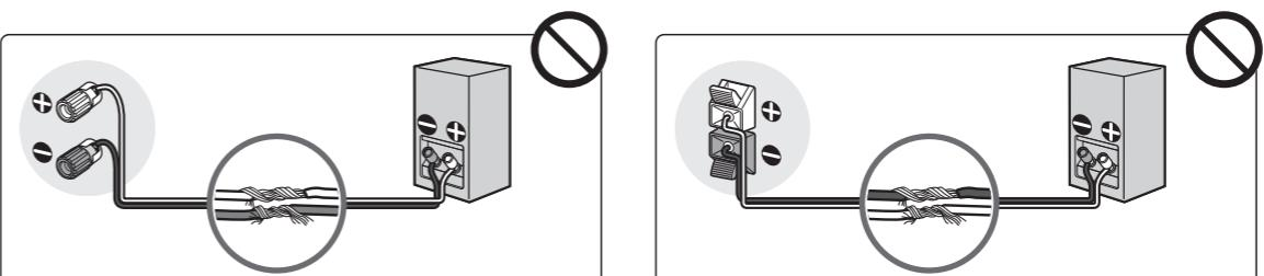
Do not connect two speaker cables to lengthen it.
