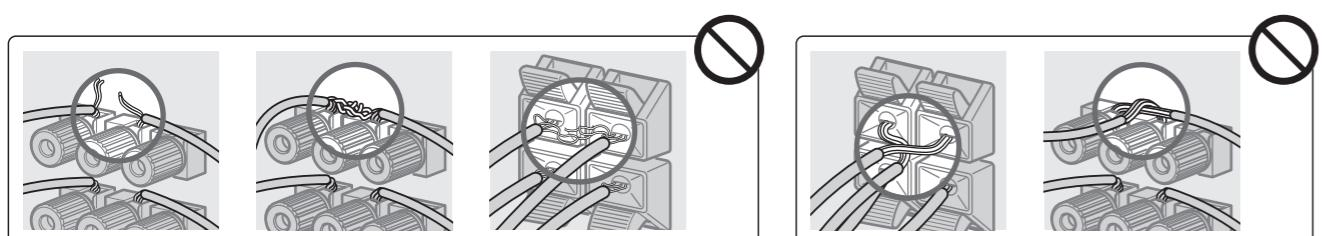
Stripped speaker cables are not tightly twisted and fully inserted to the speaker terminals.
