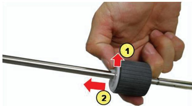
**EN** Remove the MP pick up roller while pulling the tab (callouts 1 and 2).
