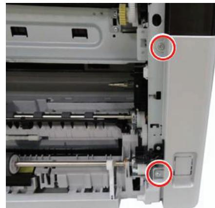
**EN** Remove two screws and then remove the rear-dummy cover.
