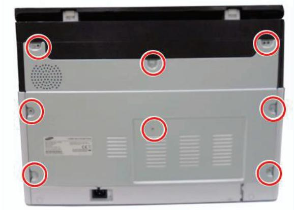
**EN** Remove eight screws and then release the rear cover.
