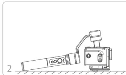
Place the gimbal on a flat, horizontal surface. The gimbal will automatically initialize after a few seconds detecting no movement. The blue light will flash three times to indicate end of initialization.
