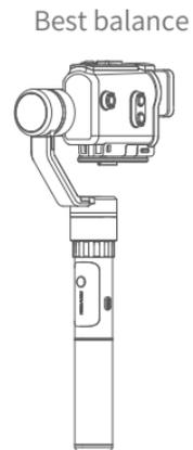
If the camera is tilted to the right, then loose camera thumb screw, move the camera to the left, try to adjust to the best balance, and then tighten the camera thumb screw.
