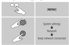
If this feature is disabled (**NO**#), the network module will be switched off whenever the radio is not actively using the network connection (such as in standby mode). This means the radio will not be accessible via the network from your PC, smartphone or tablet. You should enable (**YES** #) this menu item if you want to use streaming or control functions via the app. This function is disabled by default.
