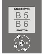
Use button © to increase the temperature = warmer (B 6 - B 9). Use button  $\oslash$  to reduce the temperature = colder (B 4 - B 1).
