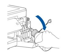
Point the nozzle upward so that the ink does not spill, and then remove the nozzle from the ink tank.
