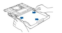
Adjust the paper guides. Fan the paper well and load it in the tray.
