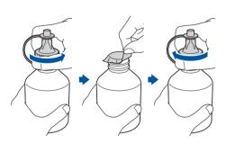
Remove the cap and protective film from the ink bottle, and then replace the cap.
