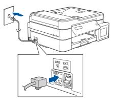
Connect the telephone line cord. Use the socket marked LINE.
