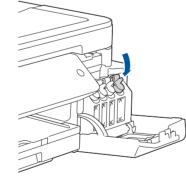
Push down on the cap of the ink tank to close it tightly. Repeat step 6 for the three other ink tanks.
