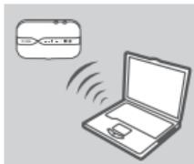
1. Use your PC's wireless adapter to connect to the **dlink\_DWR-932\_xxxx** wireless network. The wireless network name (SSID) and password are printed on the label on the battery cover.
