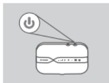
6. Press and hold the power button for three seconds to turn on the device. Once the power LED changes from green to solid blue or amber, you may proceed with configuration.
