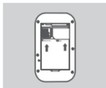
3. Slide the SIM card frame to the right and lift up. Insert the SIM/UICC card into the SIM/UICC card slot as shown, ensuring the gold contacts are facing down. Replace the frame and slide it left to lock it in position.
