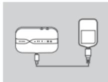
5. Connect the Micro USB end of the USB cable to the Micro USB port on the bottom of the DWR-932 and plug the USB end into the USB port of a power adapter (not included) or a PC to charge the battery.
