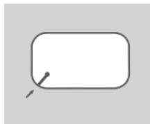
1. Remove the battery cover on the back of the device by gently prying it up from the case using the corner notch, then remove the battery.
