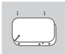
4. Reinsert the battery and replace the battery cover.
