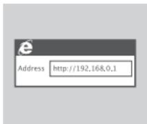
2. Use a web browser to go to **192.168.0.1** to log in to the router's configuration interface. The default username is **admin**, and the password should be left blank.
