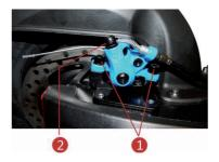
2. Remove both bolts holding the brake (1).
