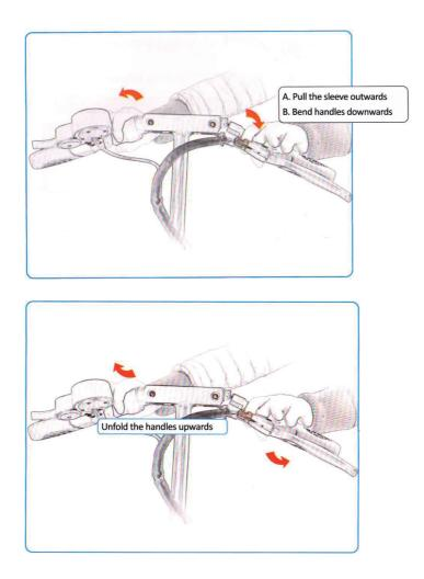
If the sleeves move rigidly, push the handles upwards while pulling the sleeves ourwards. You can also lubricate the sleeves.
