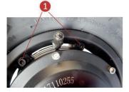
8. Remove defective / worn-out tire (inner tube) and replace it with a new one.
