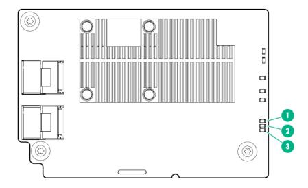
**Cache module LEDs (For standup Smart Array controllers)**
