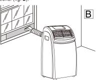
Thanks to the locking pins, it's possible to use the window bracket also for sliding windows. Position the hole of the bracket so to allow a correct installation of the exhaust hose.
