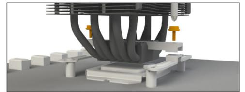
Position the cooler mounting bridge (6) centrally on the cooler (1). Next place the cooler unit onto the CPU. Insert the Intel/AMD mounting bridge fastening screws (11) from above into the cooler mounting bridge (6) and then screw these alternately tight. You can use the cross-tip screwdriver (15) for this.
