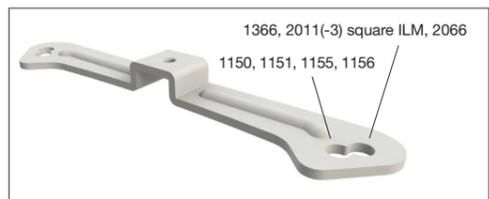
**Assembly of the cooler mounting frame**
