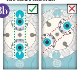
Keep turning until blue spool gaps and blue posts are lined up at the top and bottom of the machine.
