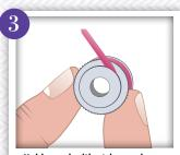
Hold spool with string end facing out.  Insert spool into spool holder until it clicks in place following the design template.
