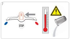
Wait until the lever moves to the "STOP" position. Extraction stops. Empty and clean container. Warning: Hot water! Handle with care!
