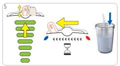
Set bar display to maximum level with selection lever. Push selection lever to the "COLD" position. Machine starts rinsing.
