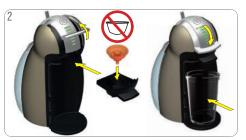
Open locking handle. Make sure that rinsing tool is in capsule holder and capsule holder is in machine. Close locking handle. Place an empty large container underneath the coffee outlet.
