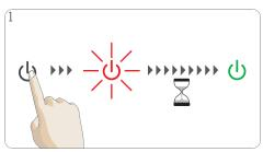
Check if the water tank contains enough fresh drinking water. Switch on machine. Power button starts blinking red while machine is heating up for approximately 40 seconds. Afterwards power button lights steady green. Machine is ready to use.
