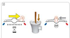
Push selection lever to the "HOT" or "COLD" position as recommended on capsule packs. Beverage preparation starts. Wait until the lever moves to the "STOP" position. Extraction stops. Extraction can be stopped manually by moving the lever back to the "STOP" position.
