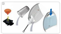
Pull out capsule holder. Remove rinsing tool. Rinse capsule holder with fresh drinking water from both sides. Reinsert capsule holder. Empty and clean container. Rinse and clean water tank. Afterwards refill with fresh drinking water and insert it into machine.
