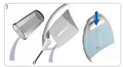
Empty and clean container. Rinse and clean water tank. Use a clean food-safe brush and washing-up liquid as needed. Afterwards refill with fresh drinking water and insert it into machine.
