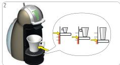
Adjust drip tray position. Place cup with correct cup size on drip tray. See 3. "BEVERAGE EXAMPLES" or package.
