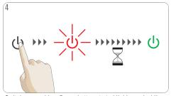
Switch on machine. Power button starts blinking red while machine is heating up for approximately 40 seconds. Afterwards power button lights steady green. Machine is ready to use.
