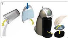
Empty container. Fill water tank with fresh drinking water. Insert water tank into machine. Place drip grid on drip tray. Then insert drip tray at desired position.
