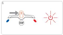
Wait until the lever moves to the "STOP" position. Extraction stops. Power button blinks red for about 5 seconds.
