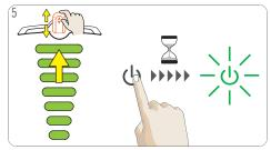
Set bar display to maximum level with selection lever. Press and hold power button for at least 5 seconds. Power button blinks green. Machine enters descaling mode.
