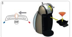
Wait until the lever moves to the "STOP" position. Open locking handle. Pull out capsule holder. Remove rinsing tool. Reinsert capsule holder.
