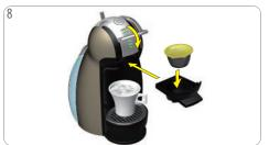
Insert second capsule in capsule holder. Insert it back into machine. Close locking handle.
