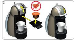
Open locking handle. Pull out capsule holder. Make sure rinsing tool is not inside. Insert first capsule in capsule holder. Insert it back into machine. Close locking handle.
