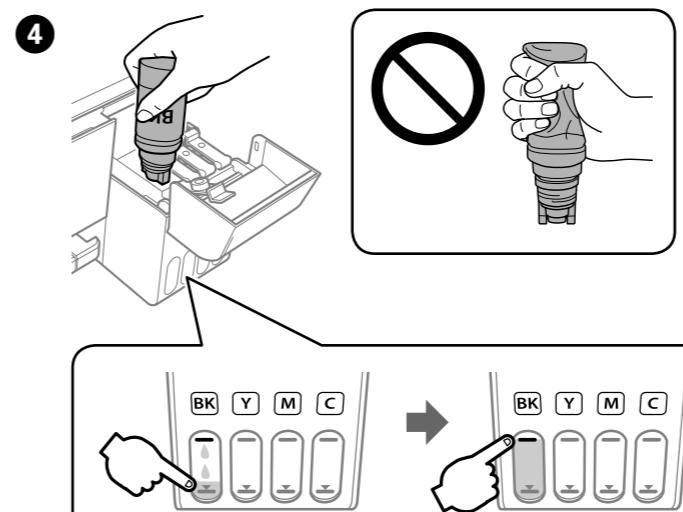
Ink flow stops automatically when the ink level reaches the upper line.
