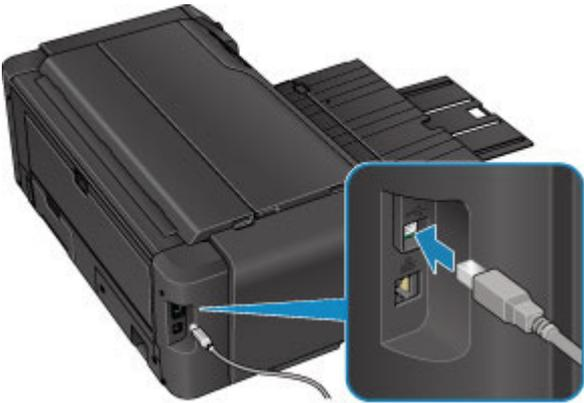
**Check2** Follow procedure below to connect printer and computer again.
