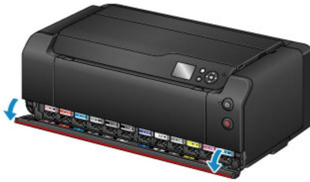
5. Remove the ink tank to be replaced.
