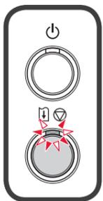
If the **Alarm** lamp flashes, check that the Print Head and ink tanks are installed correctly.
