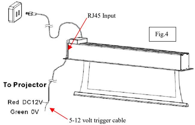
**6. Wireless 5-12 volt trigger (Item F, Fig 5):** The RF remote control serves as a dual purpose, independently as a handheld remote control, or in conjunction with the Wireless 5-12 volt trigger cable. The radio frequency technology can be programmed to send a wireless signal to synchronize its drop/rise with the projector's power cycle.
