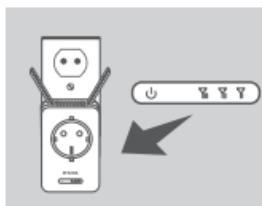
If the Signal Indicator LED has a single amber bar after the connection process has finished, the DAP-1365 has established a poor quality connection. To improve the connection quality, the DAP-1365 should be relocated to a wall outlet closer to the source wireless router or AP. The more lit bars on the Signal Indicator LED, the better the wireless signal.
