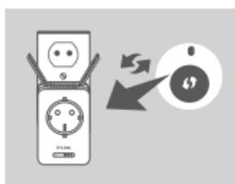
Plug the DAP-1365 into a wall outlet and wait until the Status/WPS LED is blinking amber. Push the WPS button on the source wireless router or AP, and then push the WPS button on the side of the DAP-1365. The Status/WPS LED will start to flash green.
