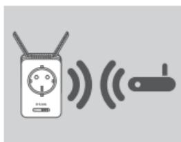
Please allow up to two minutes for the process to finish. The Status/WPS LED will turn solid green when the DAP-1365 has connected successfully to the source wireless router or AP.
