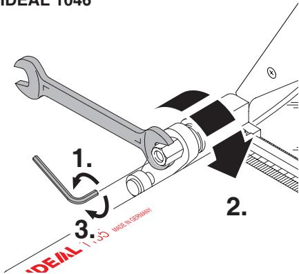
**EN** The machine has a **friction device** on the knife carrier. This insures, that the knife carrier cannot move down on its own. If it does re-adjust the friction device as follows:
