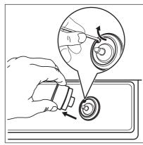
With a thin screwdriver, adjust the bypass screw position (A).
