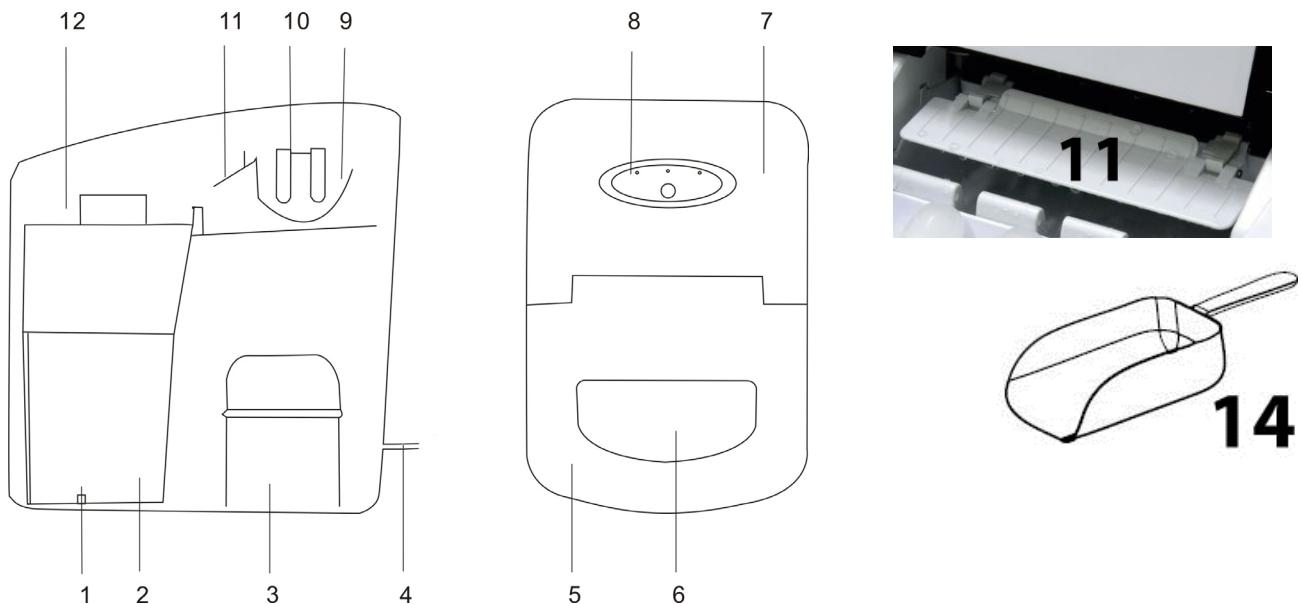
1 water outlet with silicon plug (pull it from the inside)
