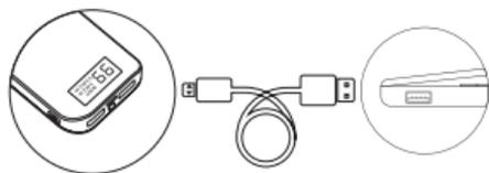
Connect the powerbank to a free USB port on a computer with the supplied USB to Micro-USB cable directly.
