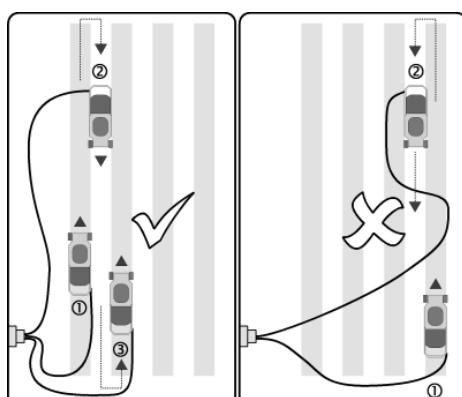
**Warning:** Do not mowe towards the cable as shown in right picture.
