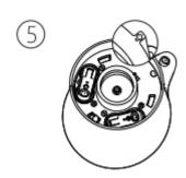
Align the unlocking mark on the battery cover with the arrow mark on the side wall of the fuselage
