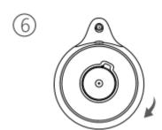
Rotate the battery cover clockwise with the lock mark aligned with the arrow mark on the side wall of the fuselage
