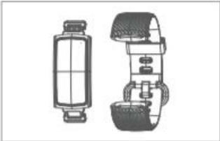
Charging the battery: Insert the chip-mounted end of the bracelet body into the USB interface to activate the product by charging (be cautious to not reverse the polarity, and comply with the required voltage and current: 5V / 500mA)
