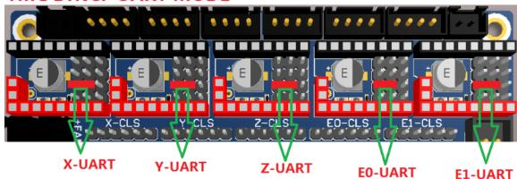
Note: When using the TMC2209, if you can't use the stallguard function, you need to cut off the DIAG pin on the driver so that the mechanical switch can work normally. The operation method is as shown below:
