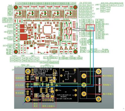
6. The connection of SKR V1.4 and Resume Printing While Power Off Module (UPS  $24V\ V1.0$ ) :
