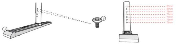
STEP 5: Install the USB Hub and Headset Hook on the metallic panel and fix it in place using one M6 wide head screw (choose your desired direction).
