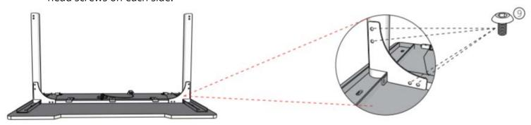
STEP 3: Fix the table legs onto the desktop using four M6 wide head cap screws on each side.
