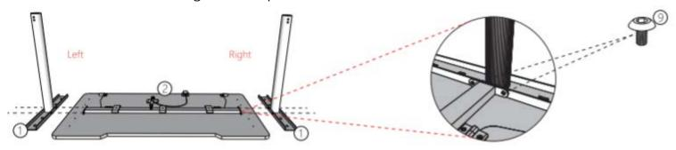
STEP 2: Install the metallic stator on the table legs and the crossbeam using four M6 cup head screws on each side.
