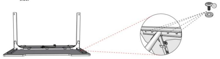
STEP 4: (Pre-installed) Insert the footing into the table leg, after which fix the footing to the required height using two M8 wide head screws on each side (there are 7 height options in total).
