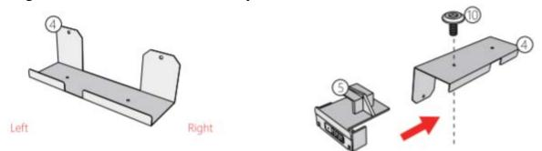
STEP 6: Fix the metallic panel onto the table legs using two M6 cup head screws. Choose the same side as your computer.
