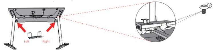
STEP 7: Lock all the fixing screws in place, turn the table over, and nip the 3 cable management clips to complete the installation. Choose your desired direction
