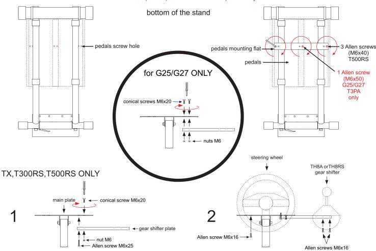
Drive 1 conical screw (M6x20) and 1 nut M6 to connect the gear shifter plate with the main plate. Next put your wheel on the main plate and drive 1 Allen screw (M6x25) from the bottom to connect the steering wheel with the main plate and the gear shifter plate - TX, T300RS and T500RS only (seeT500RS set up video)
