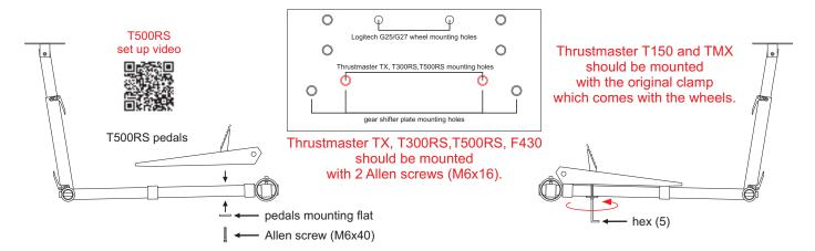
Put your pedals in the centre of the stand and drive 3 Allen screws (M6x40) to fix it firmly.
