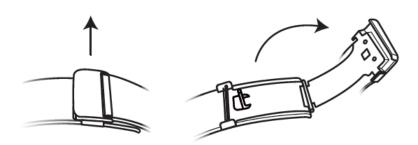
2. Pull the bottom plate upward so it is at a 90° angle with the strap.
