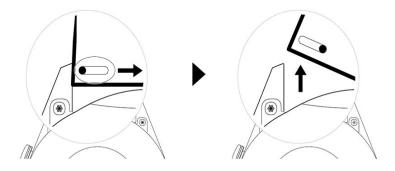
To remove a metal strap, perform the steps shown in the following figure. Follow the steps in the reverse order to install a new strap.
