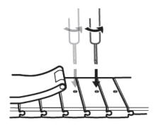
2. Remove a link from both sides of the clasp to make sure the watch face is still centered.
