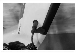
Please notice there is a charging hole in the frame, battery can be charged directly in the bike.
