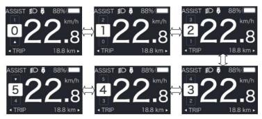
Note: if the controller has Boost function, can be selected this level with briefly press ...
