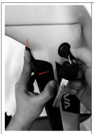
Open the lock, push up the handle with index finger, and pull down the battery for a while
