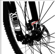
Take out the front wheel set and align it with the clearance of the front brake before installing it, then install.
