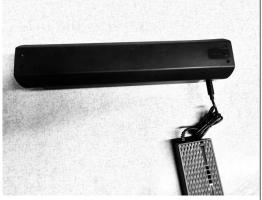
You can also take the battery out of the frame and charge the battery directly .
