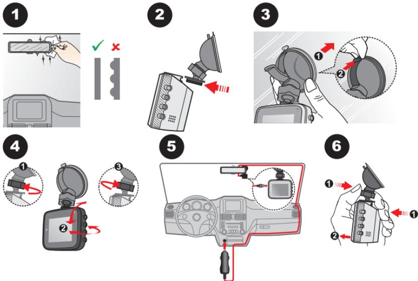
Use cable clips to secure the power cord so that it does not interfere with driving. To ensure the highest quality recordings, you are advised to place your Mio near the rear view mirror.
