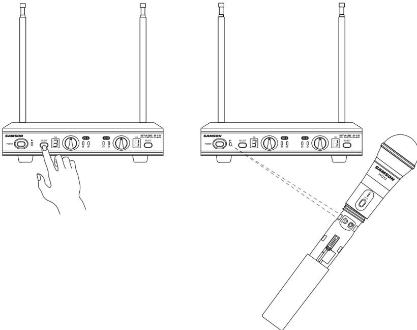
When the transmission is complete, the SR212 will receive RF signal and the tone key from the transmitter. The CH A READY indicator will light on the front panel of the SR212 receiver. Repeat these steps for the CH B transmitter and receiver. CH A and CH B available frequency channels do not overlap, so you can set the two receivers to the same channel number or letter.
