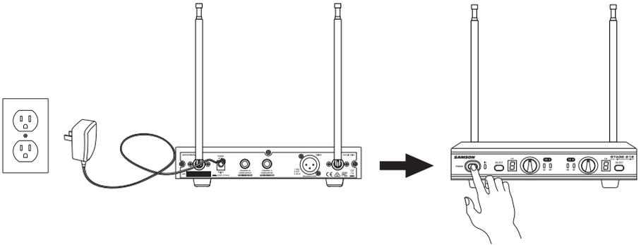
With your amplifier or mixer off and volume control all the way down, connect the SR212 receiver 1/4" outputs (or XLR Mix Output) to the inputs of a mixer or amplifier. Turn the Level knob on the SR212 completely counterclockwise, then turn its power on.
