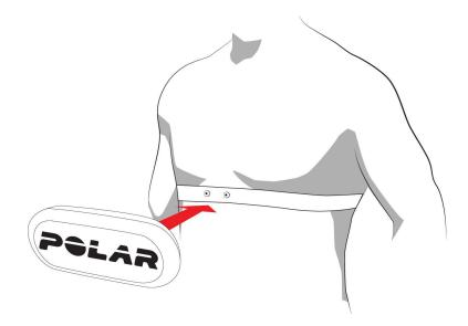
Detach the connector from the strap and rinse the strap under running water after every use. Sweat and moisture may keep the electrodes wet and the heart rate sensor activated. This will reduce the transmitter battery life.
