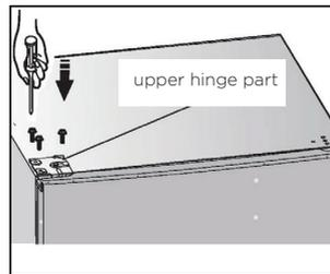
11. Install the screw hole cover on the top right corner of the refrigerator. Install the upper hinge cover (which is in the plastic bag) on the left corner. Put the other upper hinge cover into the plastic bag.
