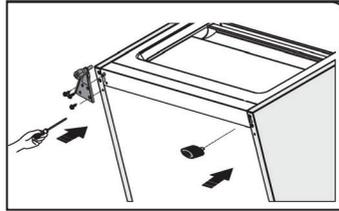
9. Transfer the door to the property position, adjust the lower hinge part, make the hinge axis into the lower hole of the door.
