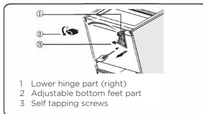
8. Replace the lower hinge part to the left side and fixing it with the special flange self-tapping screws. Replace the adjustable bottom feet parts to another side and fixing it.
