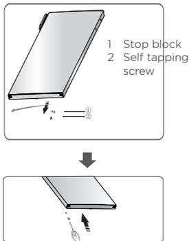
7. Lay the refrigerator on soft foam packaging or similar material. Remove both adjustable bottom feet parts, and the lower hinge part by unscrewing the special flange self-tapping screws.
