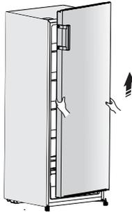
6. Place the upper door on a smooth surface with its panel upwards. Loose screw (2) and part (1), then install them to the left side and tighten securely.
