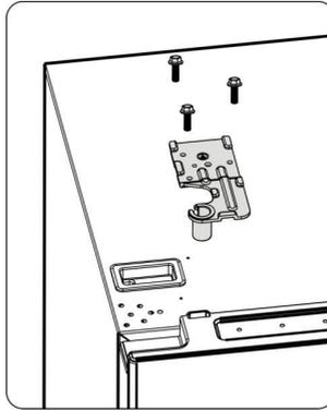
4. Open the freezer door for a small angle, then lift it up with both hands and take it off. Be careful of racks while remove the door.
