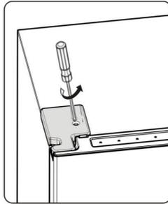
2. Disconnect terminal, open the door totally and take down upper hinge cover. Then close the door.
