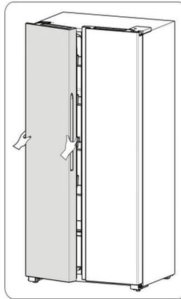
5. Remove all shelves and drawers inside the appliance. Tip the refrigerator backwards, remove the screws fixed on the hinge with a Wrench. Then remove the lower hinge.
