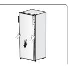
9 .Transfer the upper hinge part and make the upper hinge axis into the upper hole of the door, and adjust the position of the door (please support the door with your hand when doing it), fixing the upper hinge part with the special flange self-tapping screws.
