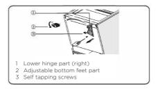
7. Replace the lower hinge part to the left side and fixing it with the special flange self-tapping screws. Replace the adjustable bottom feet parts to another side and fixing it.
