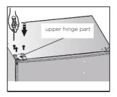
10.Install the screw hole cover on the top right corner of the appliance. Install the upper hinge cover (which is in the plastic bag) on the left corner. Put the other upper hinge cover into the plastic bag.
