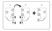
4.Remove the door from the lower hinge.
