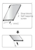
6.Lay the appliance on soft foam packaging or similar material. Remove both adjustable bottom feet parts, and the lower hinge part by unscrewing the special flange self-tapping screws.
