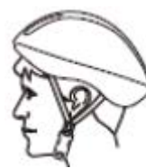
Incorrect Forehead Exposed
