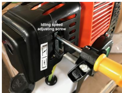
(1): Idling speed adjusting screw (cross screw)
