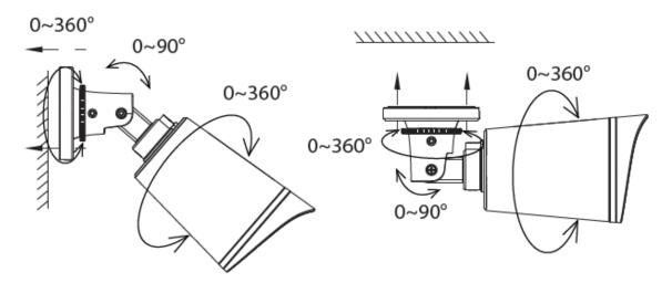
Point the camera at the desired location and use the screws provided to mount it.
