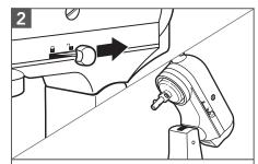
Unlock and lift the Motor Head. Then, lock\*\* the head to keep it lifted.
