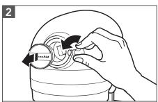
Loosen attachment knob by turning it counterclockwise. Remove attachment hub cover.
