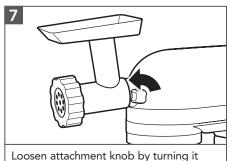
counterclockwise. Rotate attachment slightly back and forth while pulling out.
