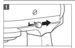
To lift motor head: Push the locking lever to the UNLOCK position and lift the head. Once lifted, the lever will automatically go back in LOCK position to keep the head lifted.
