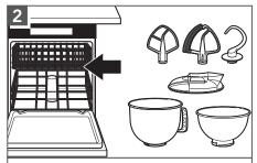
Bowl, Pouring Shield\*, white Flat Beater, Flex Edge Beater\*, and white Dough Hook may be washed in a dishwasher. Or, clean them thoroughly in hot sudsy water and rinse completely before drying. Do not store beaters on shaft.
