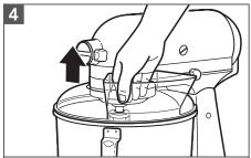
Lift the front of the Pouring Shield clear of the Bowl rim and pull forward. Remove attachment and Bowl.
