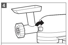
Tighten attachment knob by turning clockwise until attachment is completely secured to Stand Mixer. Plug into proper electrical outlet.
