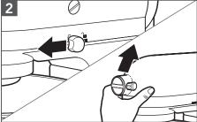
To put down motor head: Push the locking lever to UNLOCK and gently bring the head down. The locking lever will automatically go back in LOCK position when the head is down. Before mixing, test lock by attempting to raise motor head.
