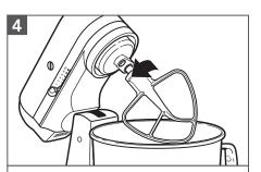
**To remove accessory:** Repeat steps 1 and 2. Press accessory upward as far as possible and turn to the left. Then pull accessory from the beater shaft.
