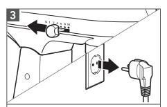
**To remove Pouring Shield:** Turn speed control to "0". Unplug Stand Mixer.
