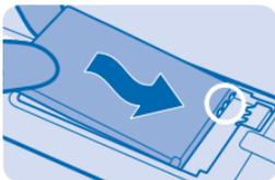
5. Replace the back cover, and press it down until it locks into place.
