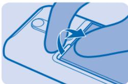
3. Slide the SIM into the holder with the contact area face down. To insert a second SIM, slide it into the other holder .
