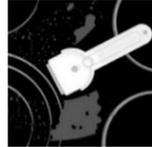
Remove stubborn and burnt residues with a scraper. Be careful when handling the scraper to prevent injury.
