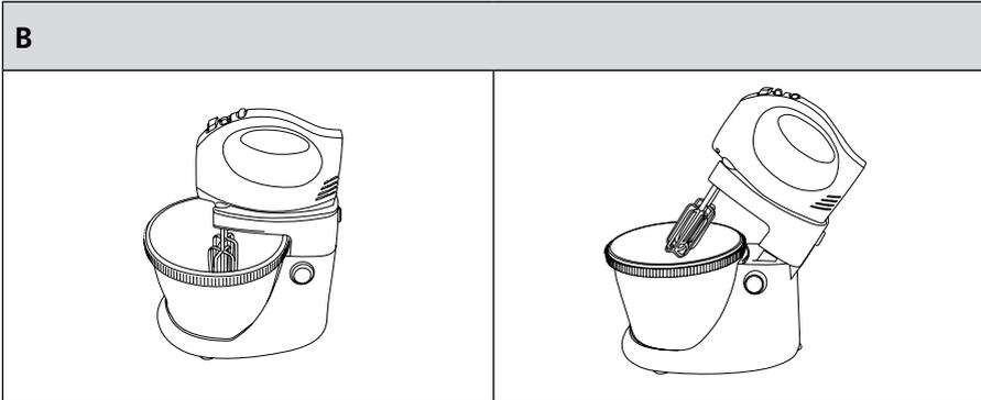
Press button ⑩ to release the lock of the motor unit ⑦ and with the other hand remove the motor unit ⑦. To release the attachments press button ③ and remove the attachments.
